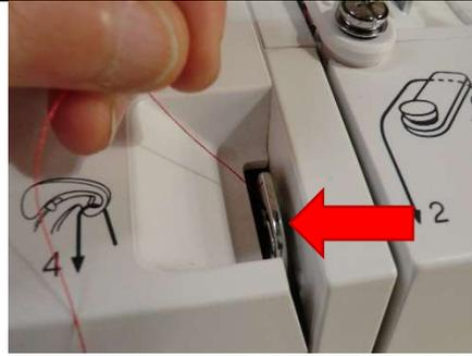
**Step 7: Bring the thread through the lower thread guide**
