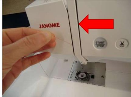
**Step 6: Pass the thread through the eye of the take-up lever**
