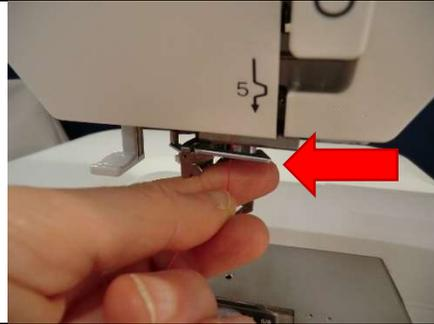
**Step 8: Bring the thread through the needle bar thread guide**
