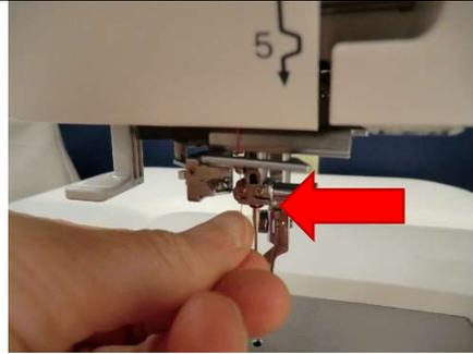
**Step 9: Use the thread cutter to trim the thread to length**
